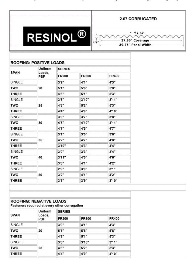
Complex Plastics Inc. Resinol Span Panel Load - Span Tables - fiberglass corrugated panels
