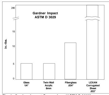
Fig. 4. Gardner Impact Comparison (ASTM D 3029)
