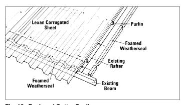
Fig. 10. Peak and Gutter Sealing
