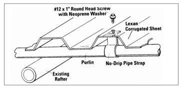
Fig. 13. Fastening to Purlin with "No-Drip" Pipe Strap
