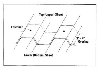
Fig. 6. Horizontal Overlapping Sheets
