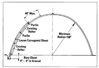
Fig. 5. Bending/Burying Lexan Corrugated Sheet
