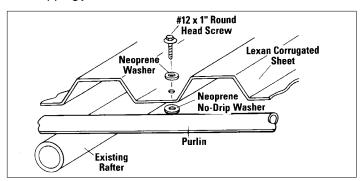
Fig. 11. Fastening to Purlin with "No Drip" Spacer
