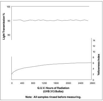
Fig. 2. LEXAN Corrugated Sheet Accelerated Weathering
