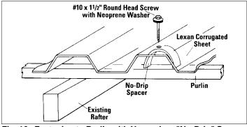
Fig. 12. Fastening to Purlin with Horseshoe "No-Drip" Spacer
