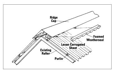
Fig. 9. Ridge Sealing
