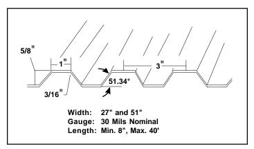
Fig. 1. LEXAN Corrugated Sheet Profile and Dimensions
