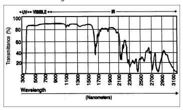
Fig. 3. LEXAN Corrugated Sheet Wavelength Transmission
